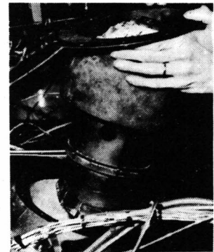
FIG. 19: ASSEMBLY OF AN EXPERIMENTAL COMBUSTOR INTO MTU-TRUCK TURBINE (1977)
